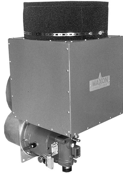
Air filter assemblies help to trap airborne particulate matter. They are offered with washable replaceable filter elements or with permanent metallic elements (as shown in photograph above). Filters mount onto OVENPAK® Burner's blower housing (or silencer housing of burners so equipped) and surround the blower motor and combustion air inlet.
