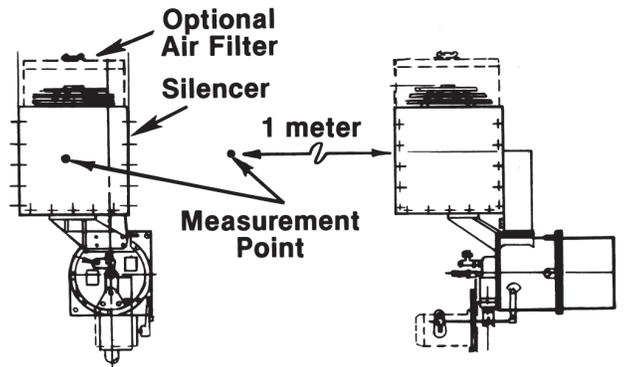
Filter silencers help reduce noise levels. They mount onto OVENPAK® Burner's blower housing and enclose the blower motor and combustion air inlet (as shown in above photograph). They can be furnished in conjunction with a permanent or replaceable filter element assembly described above.
