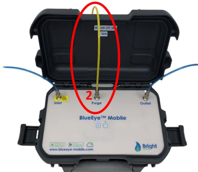
Connecting the "PURGE" allows to purge the pressure regulator with a high flow rate to ensure instant measurement of the intended gas composition. On an unconstrained gas supply line, purging of the pressure regulator happens typically in less than one minute. Efficiency of purging of the pressure regulator depends on the application, the flow rate and pressure on the inlet and the time of the purge. To end the purge and start measuring, disconnect the "PURGE" tube from the BlueEye™ Mobile.
